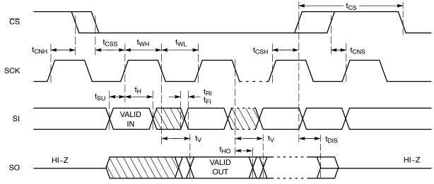
Figure 2. Synchronous Data Timing
