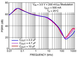
Figure 10. PSRR vs. Frequency & Output Capacitor
