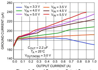
Figure 6. Ground Current vs. Output Current
