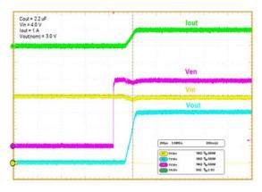
Figure 14. Turn-on by Enable Signal
