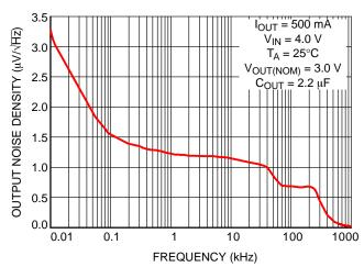
Figure 12. Output Noise Density vs. Frequency
