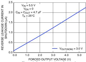
Figure 9. Reverse Leakage Current in Shutdown
