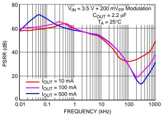
Figure 11. PSRR vs. Frequency & Output Current
