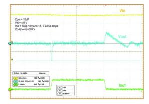
Figure 16. Load Transient Response
