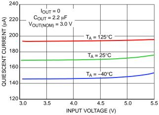
Figure 5. Quiescent Current vs. Input Voltage
