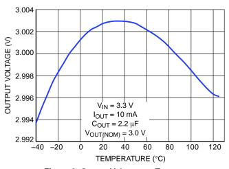
Figure 3. Output Voltage vs. Temperature
