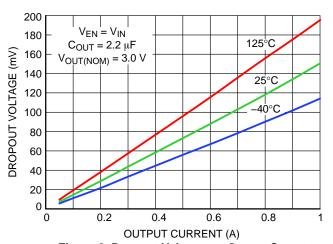
Figure 8. Dropout Voltage vs. Output Current
