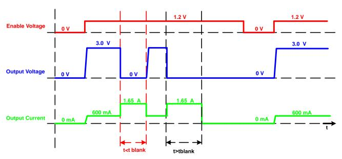
Figure 18. Overcurrent Latch Operation
