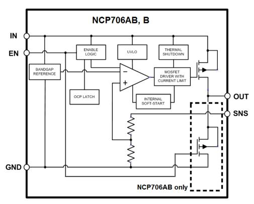
Figure 2. Simplified Internal Schematic Block Diagram
