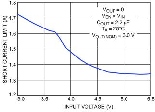
Figure 7. Short Current Limitation vs. Input Voltage
