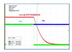
Figure 17. Turn-off by Enable Signal
