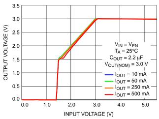
Figure 4. Output Voltage vs. Input Voltage
