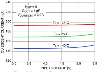
Figure 5. Quiescent Current vs. Input Voltage
