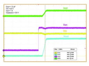
Figure 14. Turn-on by Enable Signal
