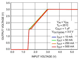
Figure 4. Output Voltage vs. Input Voltage
