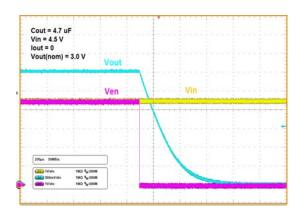
Figure 17. Turn-off by Enable Signal
