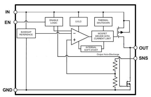
Figure 2. Simplified Internal Schematic Block Diagram
