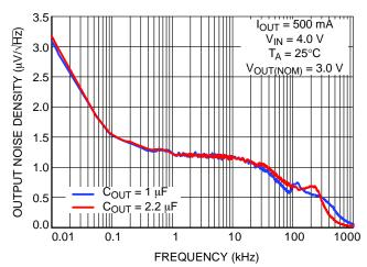
Figure 12. Output Noise Density vs. Frequency
