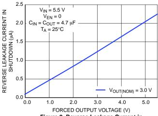
Figure 9. Reverse Leakage Current in Shutdown
