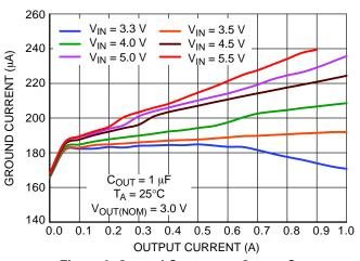
Figure 6. Ground Current vs. Output Current
