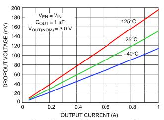
Figure 8. Dropout Voltage vs. Output Current
