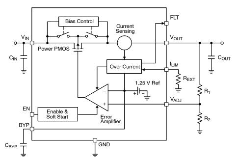
Figure 2. CAT6202 Functional Block Diagram
